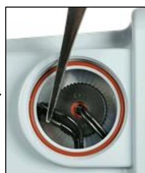
Use a tweezers to plug wire into the gap and plug in the socket
