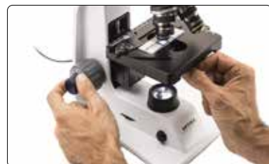
Regulation of diaphragm aperture
