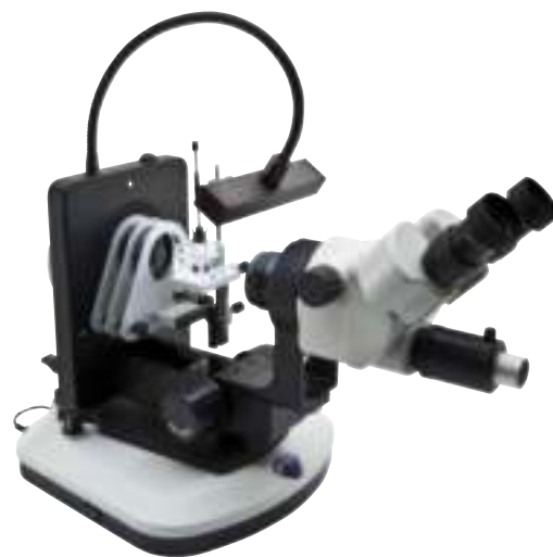
Horizontal position for immersion gem analysis
