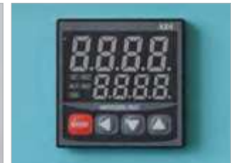
Electronic overheat protection system
