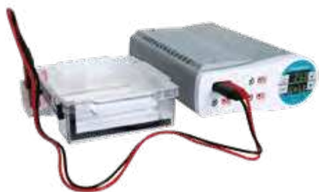
Connection to Power Supply
