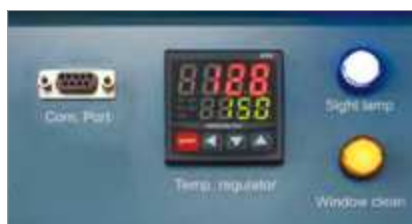
Electronic over temperature shutdown system.
