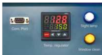
Electronic over temperature protection system.
