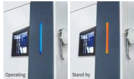
Indicator LED of operation condition
