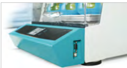
USB, RS-232 connection port provided.
