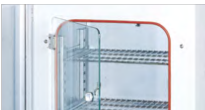
Sealed glass door for contamination prevention.
