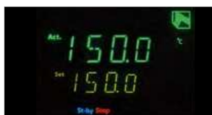
Clear VFD controller.
