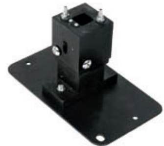
Cat. No. 18900335 10mm water-jacketed (for SCI-V1100 & SCI-UV1100)
