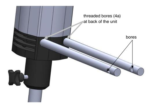
Screw the support rods (4) into the threaded bores (4a) at the back of the unit.
