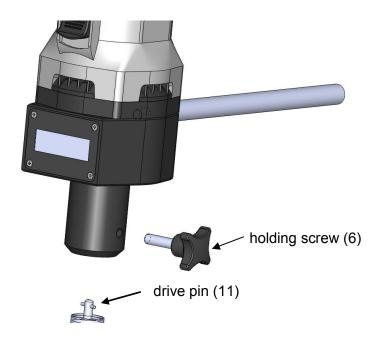
**NOTICE** Never run homogenising tools dry as the bearings and gaskets will be damaged if the generator is not cooled by the medium. The distance between the homogenising tool and the vessel bottom should not be less than 10mm. The filling of the medium may not be less than about 55 mm. To avoid a vortex it is necessary to insert the dispersing shaft out of the centre of the vessel. If these conditions are met the unit is ready for operation.
