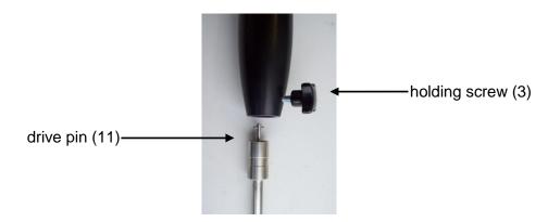
Never run a homogenising tool of type T dry as the bearings and gaskets will be damaged if the generator is not cooled by the medium. The dispersion tool must always be immersed minimum to the middle of the lower transverse bore of the shaft. The maximum immersion depth is about 3 cm below the upper transverse bore. In order not to interrupt the cooling, avoid the intake of air, or the formation of a vortex. Therefore submerge the dispersion tool deeper or eccentrically into the vessel.
