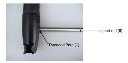
Screw the support rod (6) into the threaded bore (7) of the unit.
